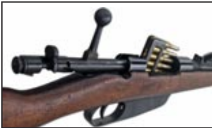
Standard infantry rifle: Carcano 91/38 held six rounds and needed the hand bolt to chamber each round.
