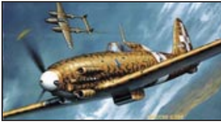
The Macchi 205 Veltro (Greyhound) one of the best fighter planes of the war, 399mph.
