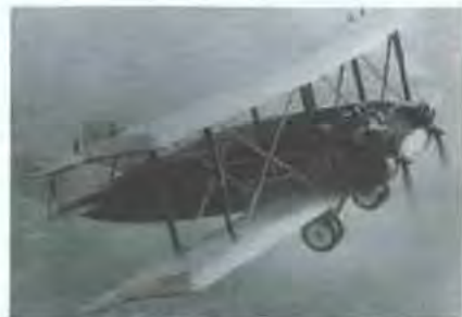
Burnelli's 1921 RB-1 was the first "lifting-body" aircraft reduced to practice.
