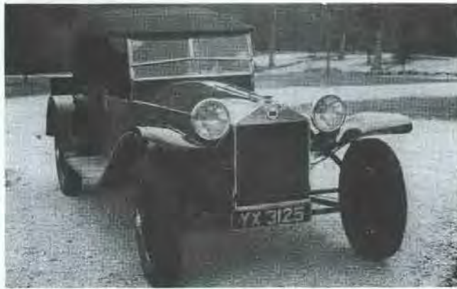
1928 Lancia Lambda Independent front suspension and unibody construction.
