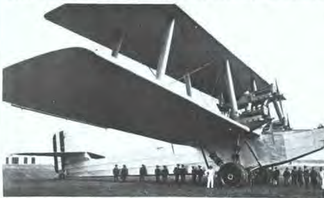
Caproni's early attempts at a mega plane. This monster was powered by six 1,000 horse power engines and could carry 11,000 pounds to an altitude of two miles.
